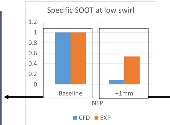
Soot mass fraction: +1mm protrusion
